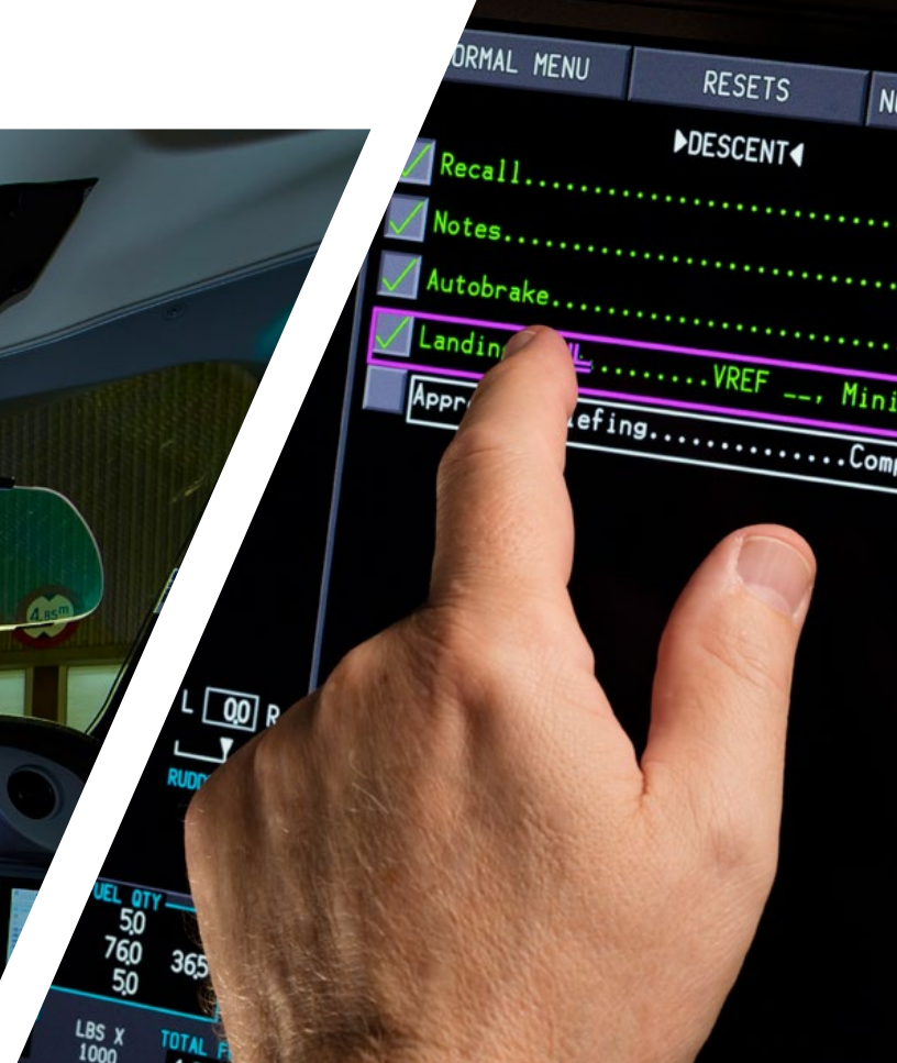
In an industry first, Boeing announced it was bringing touchscreen technology to the 777X's primary flight displays, courtesy of Rockwell Collins
