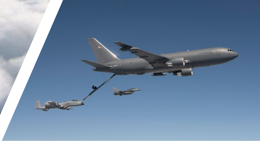
The first refueling flight for the KC-46 tanker – which also features our advanced avionics – showcased our Remote Vision System, which uses cutting-edge sensors and stereoscopic 3D displays to allow the operator to remotely control the aerial refueling boom
